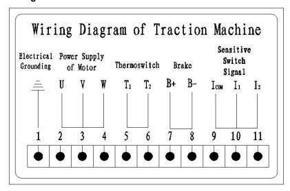
Always connect the frequency inverter output and earthing terminal to motor terminal as shown in the picture. The connection cable diameter is decided accordingly to the motor rated current (can refer to frequency inverter instruction manual).
