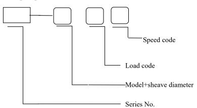
For example: CSAG-E240-1000-1.0 Type means this machine is CSAG-E gearless PMS elevator traction machine, sheave diameter is 240mm ,rated load is 1000kg, and rated speed is 1.0m/s.
