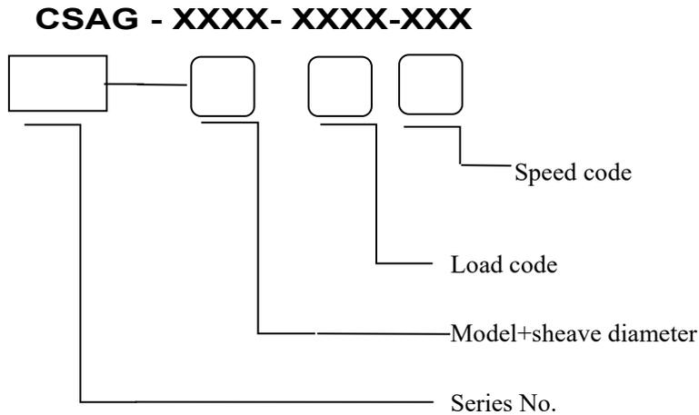
For example: CSAG-E240-1000-1.0 Type means this machine is CSAG-E gearless PMS elevator traction machine, sheave diameter is 240mm, rated load is 1000kg, and rated speed is 1.0m/s. Customer can choose our gearless PMS elevator traction machine by rated load, rated speed and series code (you can also see our gearless PMS elevator traction machine catalog for details).
