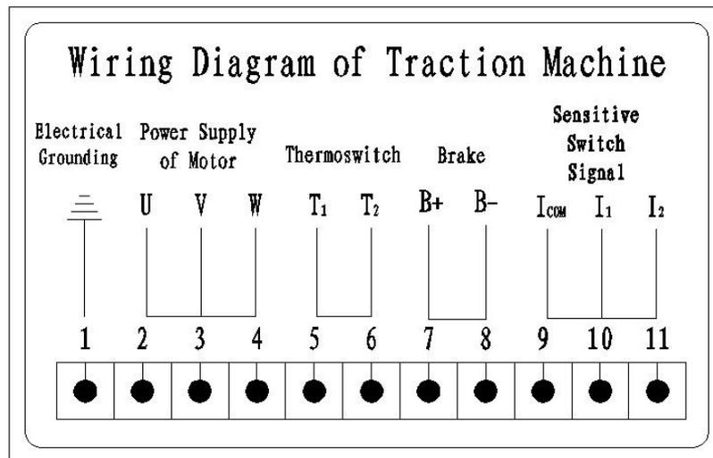
Always connect the frequency inverter output and earthing terminal to motor terminal as shown in the picture. The connection cable diameter is decided accordingly to the motor rated current (can refer to frequency inverter instruction manual).
